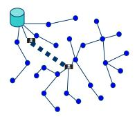
Tunnel packets received in one place of the network and replay then in another place. The attacker can have no key material. All it requires is two transceivers and one high quality out-of-band channel.
