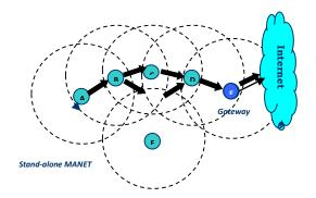
After one of the nodes is configured as a gateway, the entire network is connected to an external network like Internet *Presentation output:*
