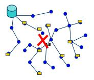
Most packets will be routed to the wormhole. The wormhole can drop packets or more subtly, selectively forward packets to avoid detection.
